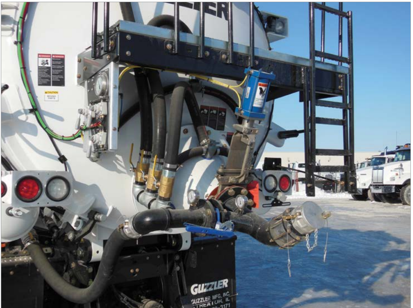
Leveraging Gardner Devner's CycloBlower, the Guzzler NX air mover is ideal for dense phase offloading applications.
