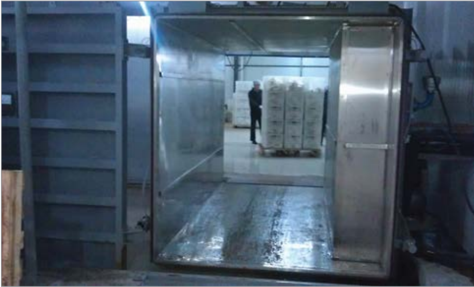
Vacuum cooling systems from ULVAC can cool two to six pallets of agricultural products per batch.
