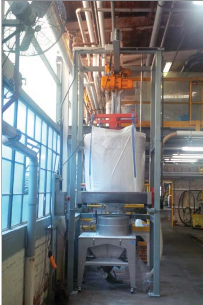
Manufactured by Volkmann, the hoist-style BBU with special loss-in-weight features helps optimize dust-free material flow.
