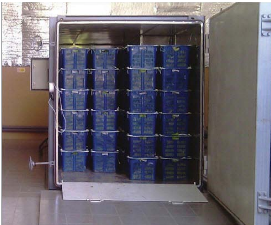
Within 20 to 30 minutes, vacuum cooling systems cool products to 39°F (4°C).
