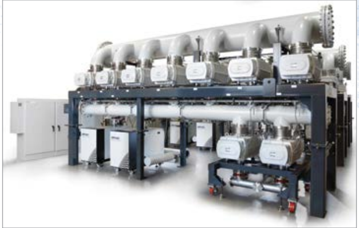
Figure 1: Steel Degassing System from Oerlikon Leybold Featuring DRYVAC® Vacuum Pumps and RUVAC boosters
