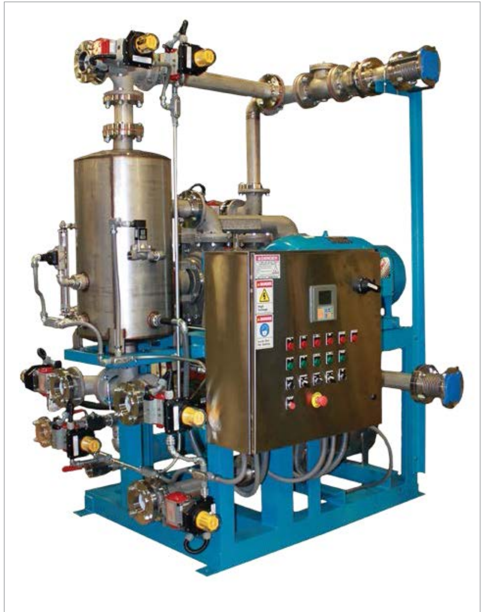
Figure 3: All stainless steel liquid ring system for beverage filling process with “clean-in-place” control system
