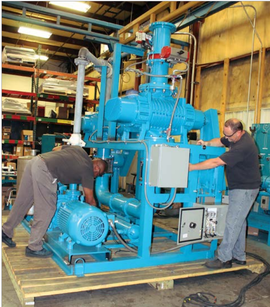
Figure 2: 3000 cfm (5100 m 3 /hr) booster/liquid ring system for plastic extrusion degassing
