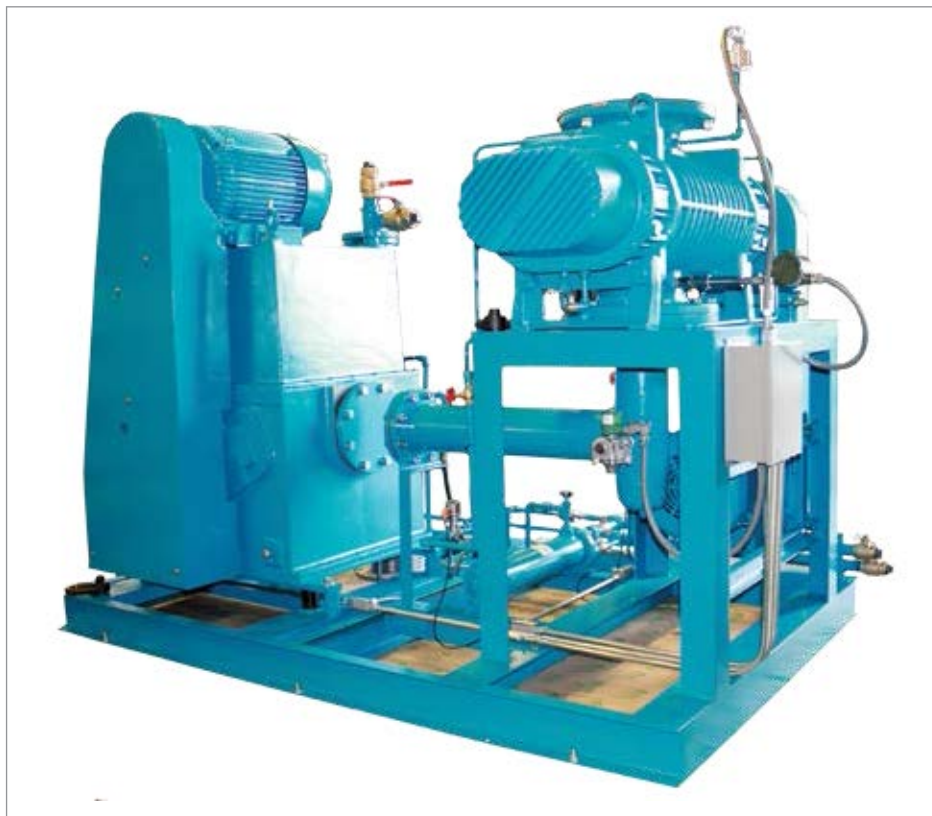
Figure 1: 4500 cfm (7650 m 3 /hr) booster/piston system for an aircraft brake pad chemical vapor deposition (CVD) furnace
