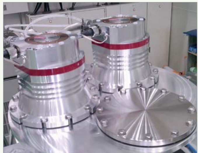
HiPace turbopumps installed at European XFEL
