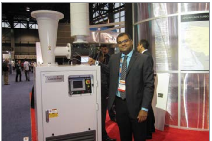
Ranjan Manivelu next to a 50 hp air bearing turbo blower at the APG-Neuros booth.
