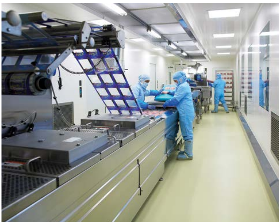
Packaging under clean room conditions: one of the packaging lines that is connected to the centralized vacuum supply.
