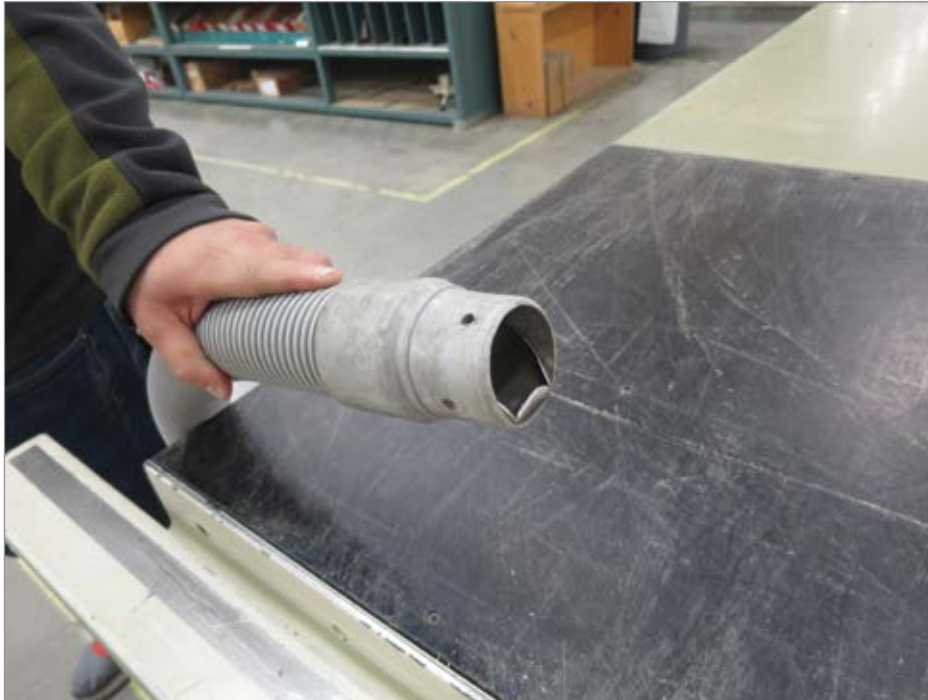
Figure 4. Typical Uncontrolled Demand at End Use – Clean-Up Wands. These types of demands are on all the time, even if the machine center is off and controlled air is off.
