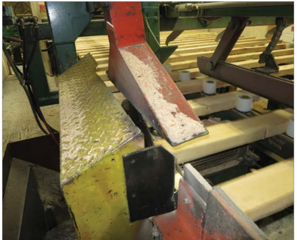
Figure 10. Poor Saw Pick-Up Point Design
