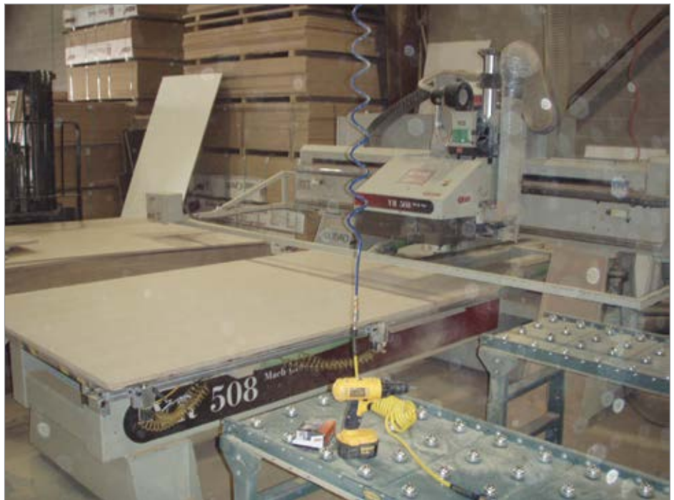
Figure 3. Typical Uncontrolled Vacuum Demand – Routing Table. The table is a porous series of tiny holes, and vacuum is always being pulled on the bottom. As larger pieces cover the table, flow decreases. So, flow is variable, not by control, but “on accident.”
