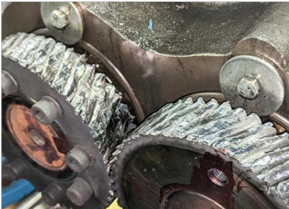
Shown is an example of gear failure from improper lubrication.
