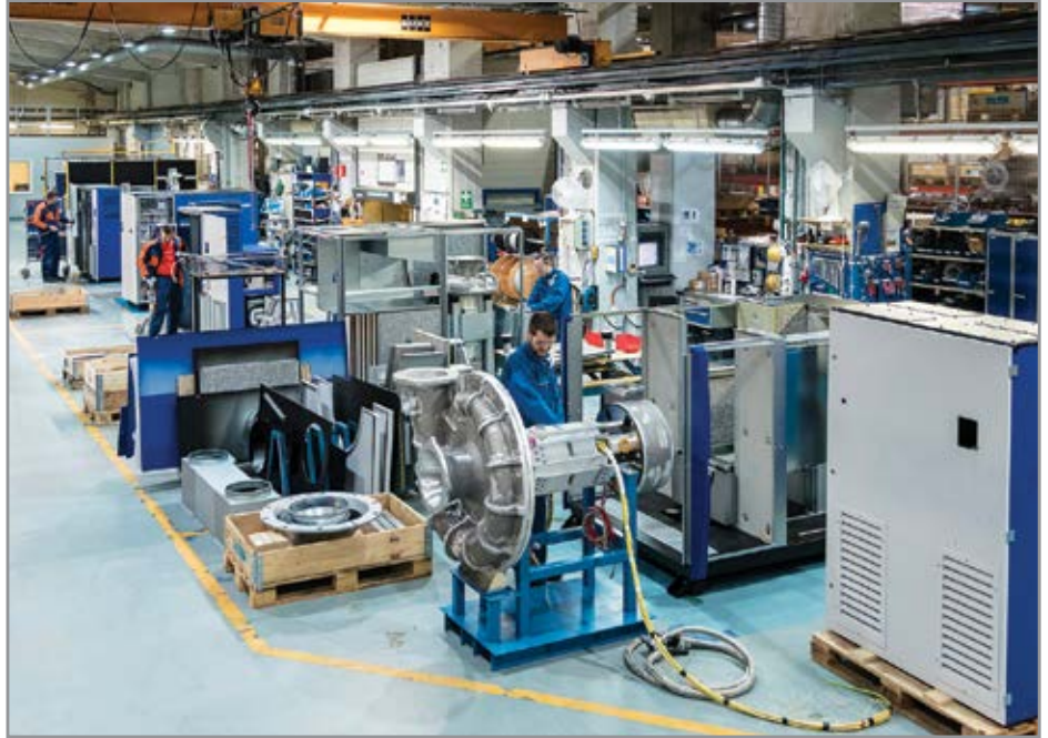
HST™ turbocompressors being manufactured in the Sulzer factory in Kotka, Finland.
