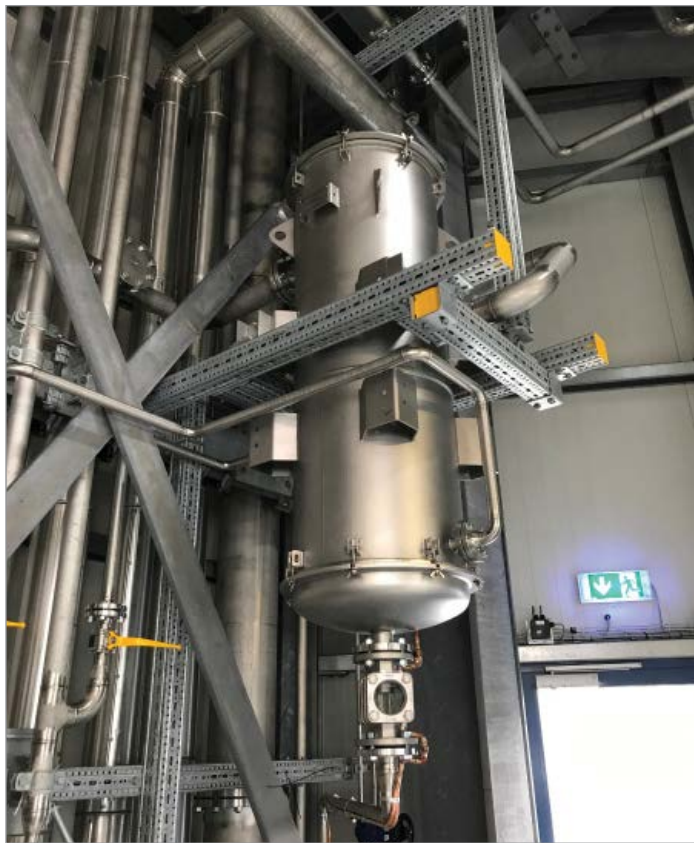
The JRS vapor condenser protects a vacuum pump from ingesting vapors given off during a plastics production process.
