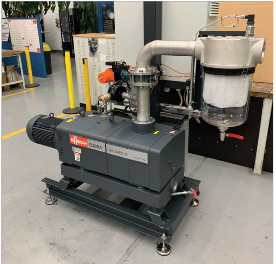
COBRA NX vacuum system for degassing clay bricks at Wienerberger.
