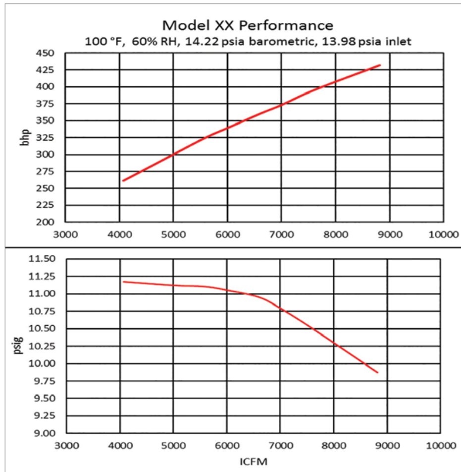
Figure 3: Example Blower Performance Curve
