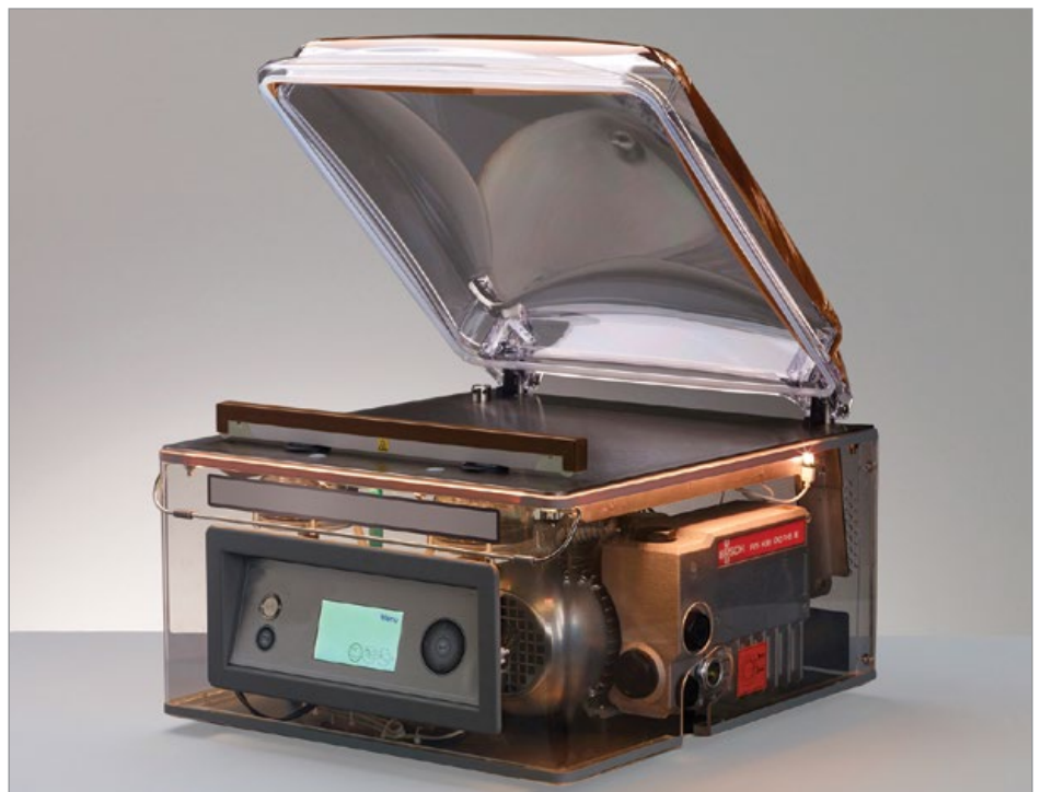
Figure 1. Functional model of a chamber packaging machine with visible rotary vane vacuum pump inside.
