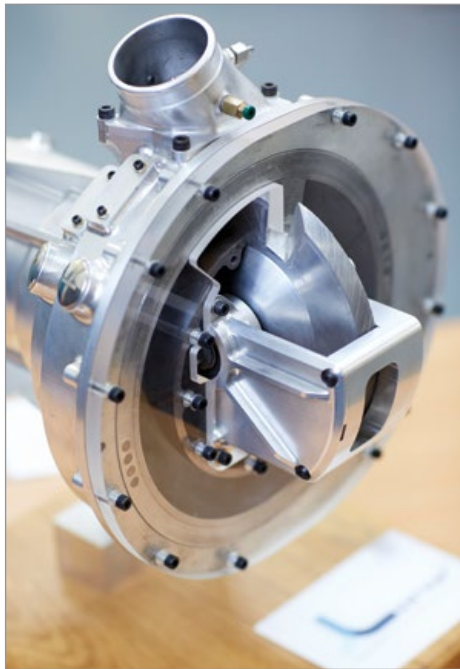
Figure 2: Internals of the LP2 blade blower from Lontra, a novel type of PD.
